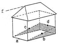
a = low point at bldg wall d=high point at bldg wallAverage Grade: (a+d)/2 = e
